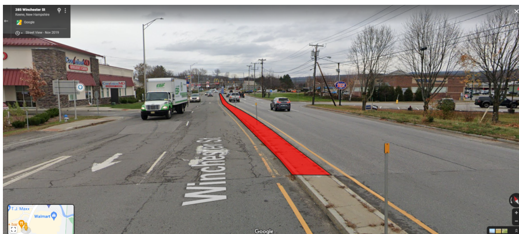
Area of median removal highlighted in red, looking north from Route 101 roundabout
